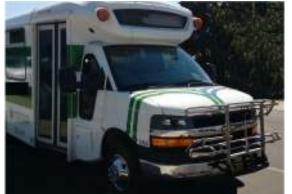
TranGO provides bike racks on all their buses. The racks hold two single seat, two-wheeled, non-motorized bicycles.
